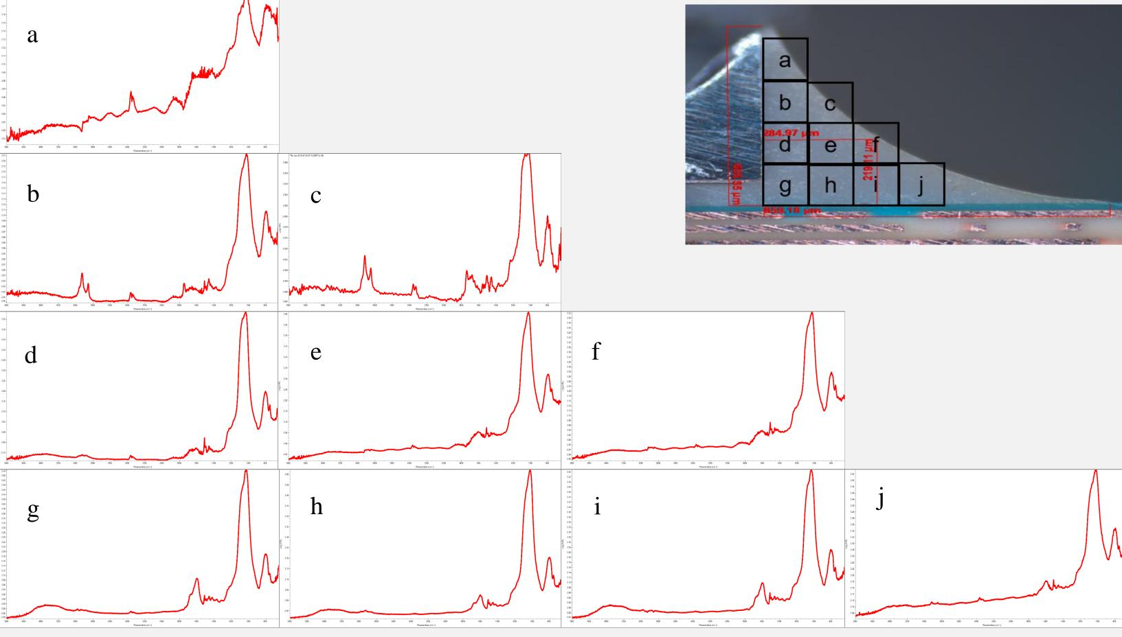
Use 150  $\mu$ m  $\times$  150  $\mu$ m working area to detect 10 different areas of sample and list as its locations.
