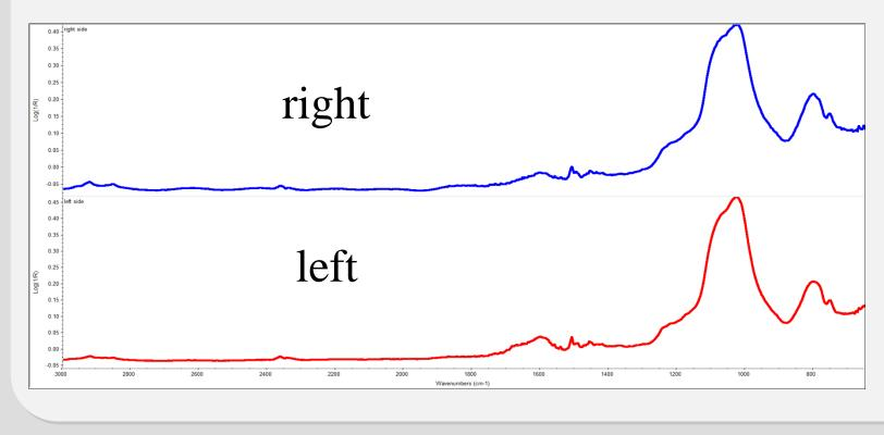
This spectrum shows the mean spectrum of both side underfill material.
