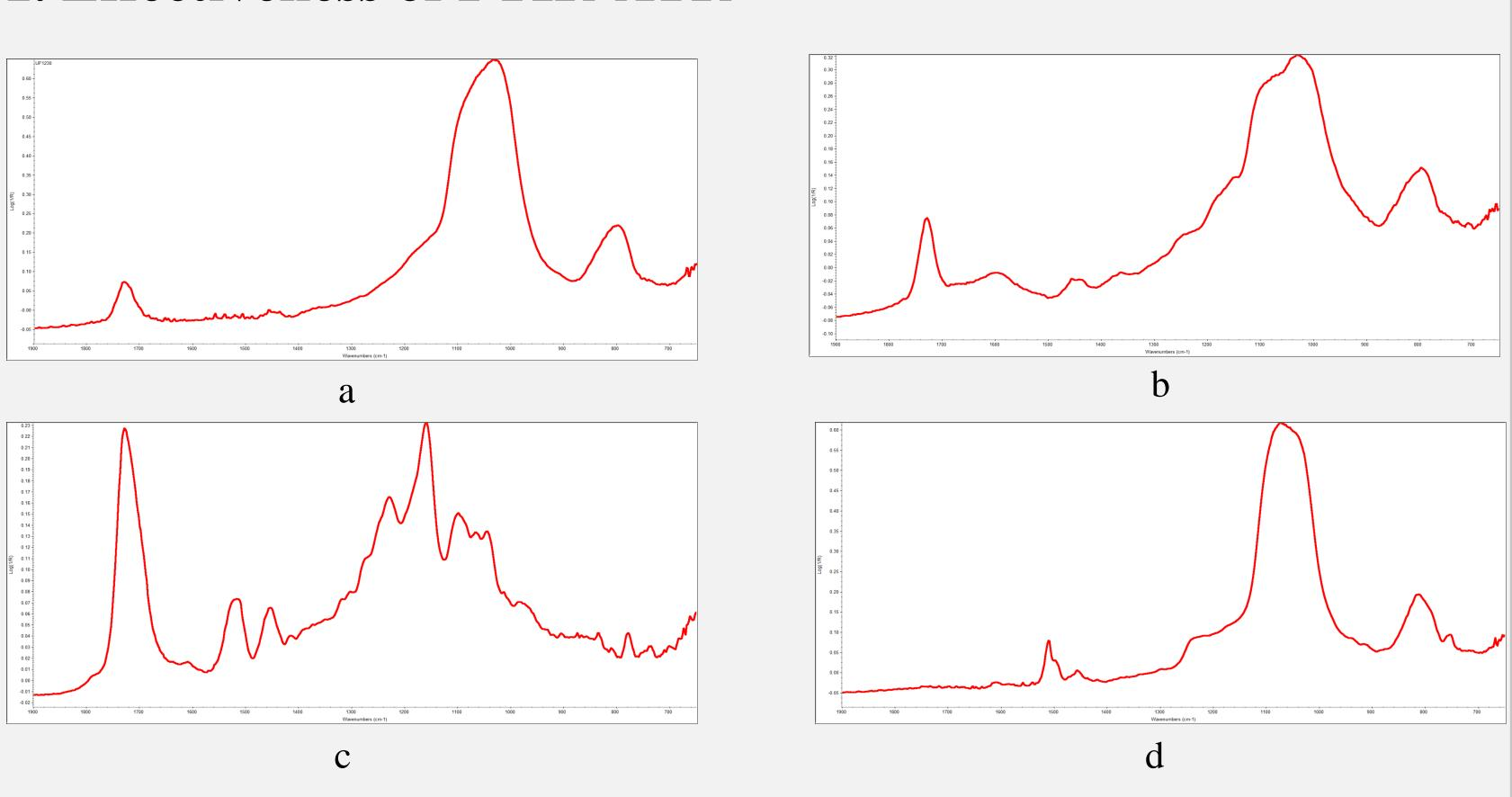
These are FTIR results of UF1230(a), EP1641(b), SMT88U(c), SMC-375TGSF5(d) four different kinds of underfill materials which UF1230 and EP1641 have similar components and similar color.
